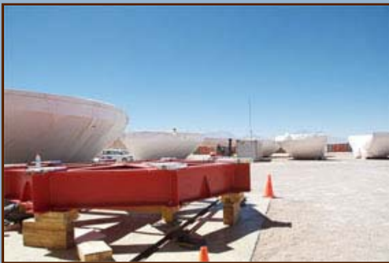
Figure 2: Antenna backup structures await assembly in the ESO/AEM contractor yard. These carbon fiber structures are shipped in halves that must be precisely glued together to form the support for the antenna panels.
