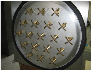
Figure: Focal L-Band Array for the Green Bank Telescope (FLAG), with 19 dual-polarized elements.
