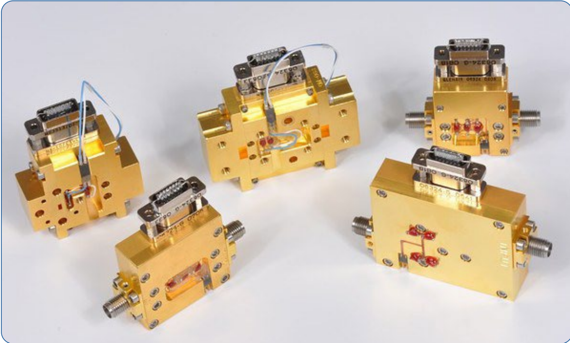
Figure: Family of cryogenic LNAs (from L-band to W-band) developed and built for the Very Large Array and Green Bank Telescope.
