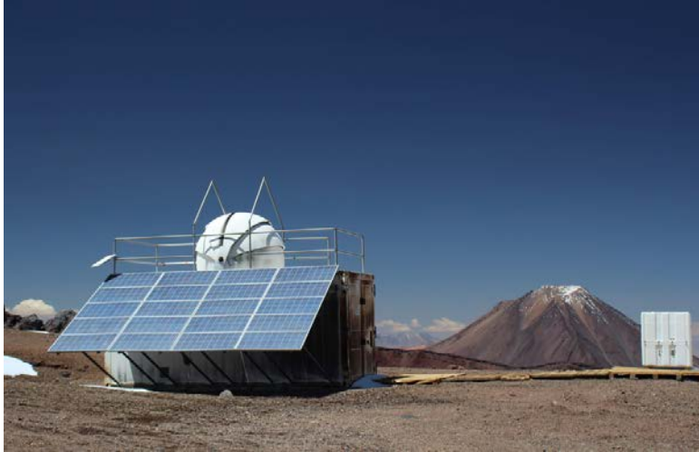
Figure B.17 The Receiver Lab Telescope (RLT) dome on top of its container. The RLT was powered by solar panels. Mounting the telescope to the ground would have required obtaining permissions that was precluded by this portable arrangement. Credit: Daniel Marrone, reproduced by permission.
