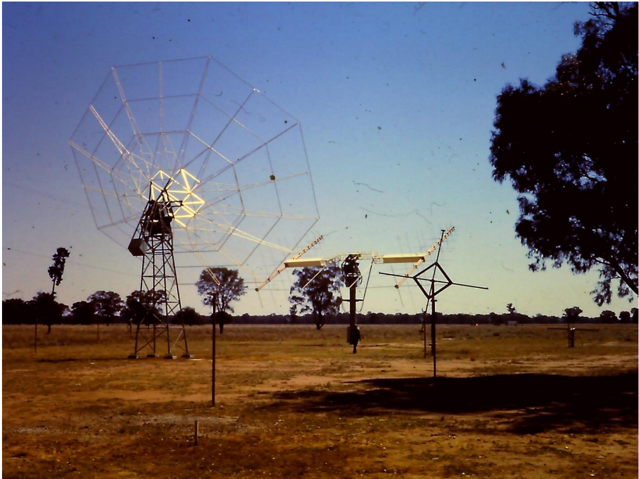
Fig 37 Photo by Goss in September 1967 at the opening of the Culgoora Radioheliograph, the 3 km diameter array consisting of 96 aerials. The figure shows one of the 13 m paraboloids of this instrument, initially operating at 80 MHz with an angular resolution of 3.8 arcmin. (Later upgrades added 43.25, 160 and 327 MHz.) The other two aerials in the foreground are radiospectrographs used to determine dynamic spectra of solar bursts. Credit: W.M. Goss
