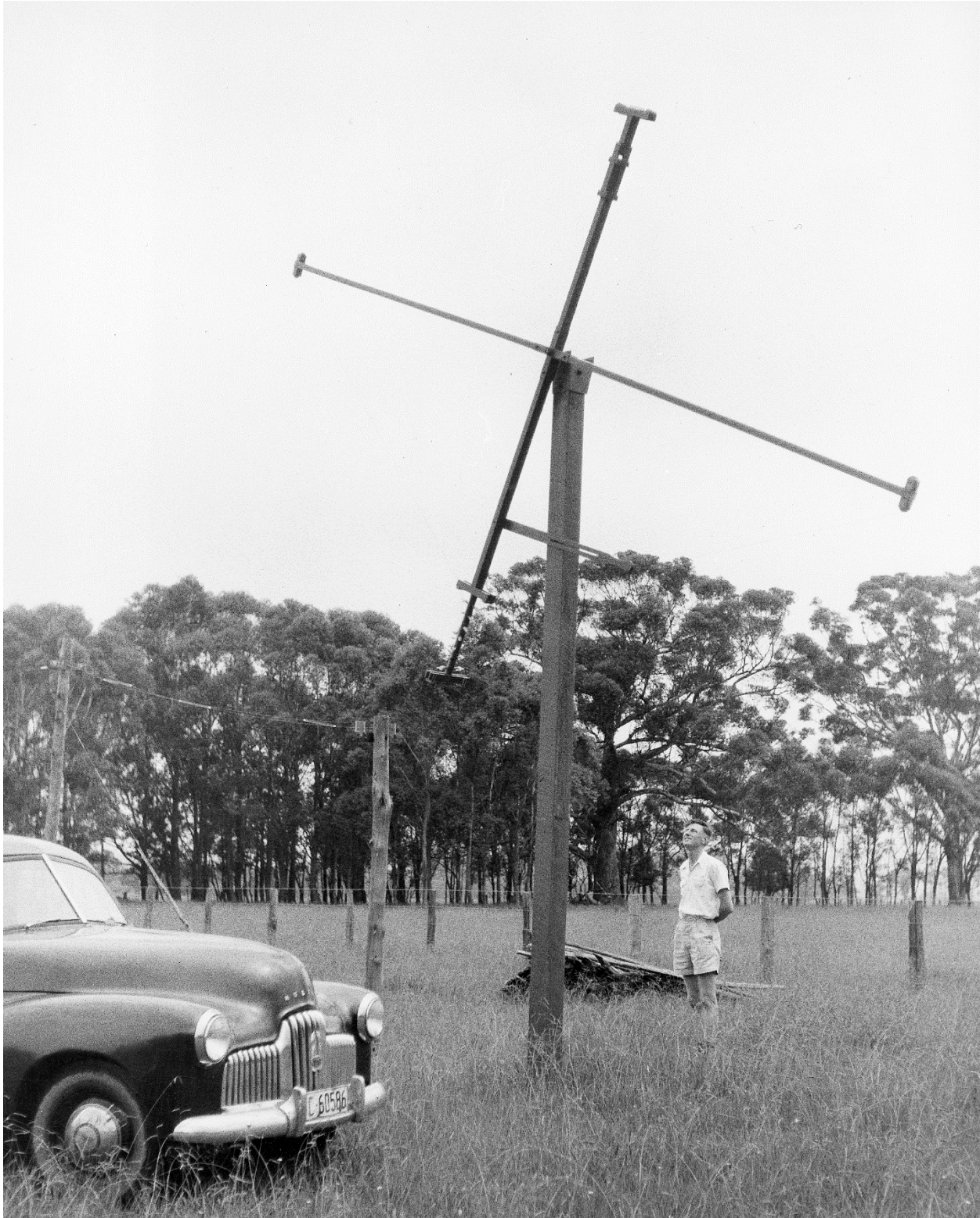
Fig. 32 Paul Wild and one of the three elements of the Dapto Swept Frequency interferometer (40 to 70 MHz). Note the open wire transmission lines used to combine the radio signals. Credit: CSIRO Radio Astronomy Image Archive R3750-2 (from 1955)
