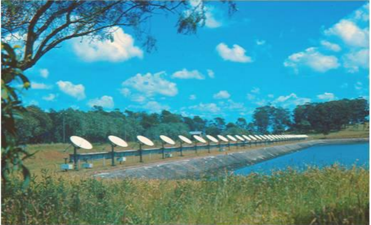
Fig. 2 A photo from circa 1953 provided by Rod Davies to Goss during a visit to Manchester, UK in May 2008. This figure shows Davies's photo of the EW grating array at 21 cm at the Potts Hill reservoir, Sydney. ©Rod Davies
