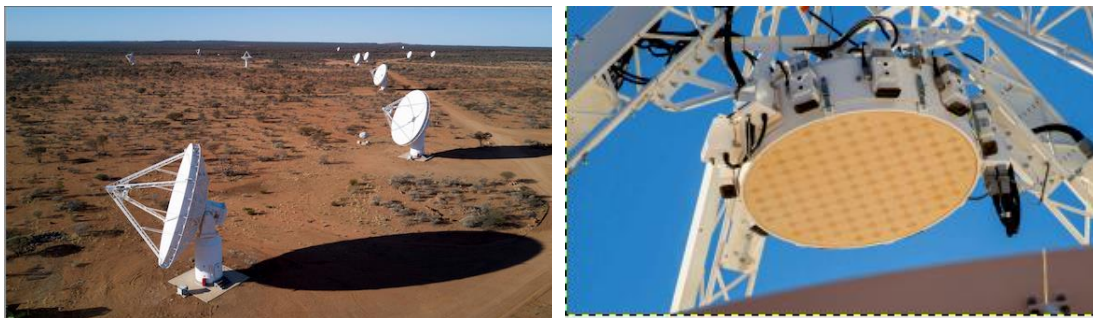
Left: antennas of the Australian SKA Pathfinder (ASKAP) at CSIRO's Murchison Radio-astronomy Observatory in Western Australia. Right: a phased-array feed on an ASKAP antenna. Credit: CSIRO
