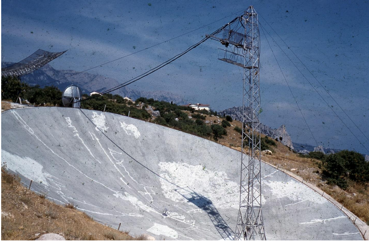
Fig. 9 Arcibo style aerial, 31 m, previously used for the ground breaking Crab Nebula polarisation detections by Arkady Kuzmin and Vyacheslav Udal'Tsov at 9.6 cm in 1957. In 1959, the latter author detected polarisation at 21 cm, with a determination of the Faraday rotation and magnetic field in the direction of the Crab Nebula based on observations of the polarisation at 21, 9.6 and 3.15 cm.
