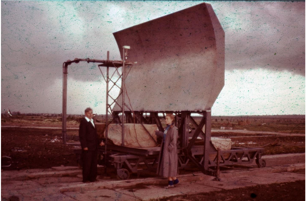
Fig. 4 Secondary reflector of BPR. Naum L. Kaidanovskii (along with Khaykin inventor of this instrument, “antenna with variable profile”) and prominent astronomer Natalya Soboleva (17 July 1935 to 1 January 2012), wife of Yuri N. Pariiskii. Leningrad branch of Special Astrophysical Observatory.
