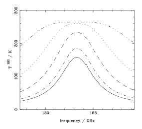
Figure 1: The effect of varying the amount of water vapour in a layer at 1km, with temperature 265 K and pressure 500 mb. Solid line is for 0.5 mm of PWV; dot-dashed for 0.675 mm; dashed for 1.275 mm; dotted, 2.8 mm; and dot-dot-dot-dashed, 6.5 mm.
