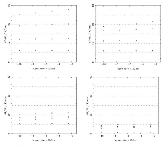
Figure 10: The effect of changing the lapse rate,  $\Gamma$ , on the radiometer channel sensitivity, dT/dL. Top left for PWV = 0.5; top right PWV = 0.675; bottom left PWV = 1.275; bottom right PWV = 2.8 mm (representing the 10,25,50 and 75 % ile frequency values). Crosses correspond to channel 1, squares to channel 2, triangles to channel 3 and circles to channel 4.
