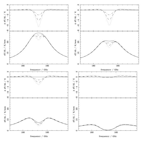
Figure 5: The effect of changing the scale height,  $h_0$ , on the brightness temperature. Top left for PWV = 0.5; top right PWV = 0.675; bottom left PWV = 1.275; bottom right PWV = 2.8 mm (representing the 10, 25, 50 and 75 % frequency values).  $h_0$  takes the values 0.5,1.0,1.5,2.0 km corresponding to solid, dot-dashed, dashed and dotted lines respectively. The top plots of each panel show the difference in brightness temperature of each line compared with the solid line.
