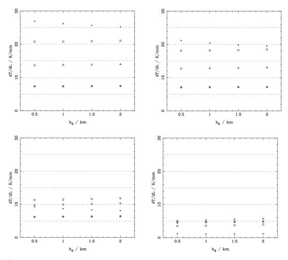
Figure 6: The effect of changing the scale height,  $h_0$ , on the radiometer channel sensitivity, dT/dL. Top left for PWV = 0.5; top right PWV = 0.675; bottom left PWV = 1.275; bottom right PWV = 2.8 mm (representing the 10,25,50 and 75 % frequency values).Crosses correspond to channel 1, squares to channel 2, triangles to channel 3 and circles to channel 4.
