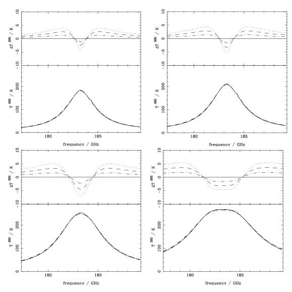
Figure 4: The effect of changing the lapse rate,  $\Gamma$ , on brightness temperature. Top left for PWV = 0.5; top right PWV = 0.675; bottom left PWV = 1.275; bottom right PWV = 2.8 mm (representing the 10,25,50 and 75 percentile frequency values).  $\Gamma$  takes values -2.5, -5, -7.5, -10.0 K/km corresponding to solid, dot-dashed, dashed and dotted lines respectively. The top plots of each panel show the difference in brightness temperature of each line compared with the solid line.
