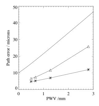
Figure 12: The predicted uncertainty in path length for a total path length of  $400\mu$ m. Stars take account only of radiometer noise (equation 15) and triangles include the dT/dL uncertainties (equation 18), with adjustments to the weights to minimise this error (table 5). The solid line shows the error specification (given by  $\{[10 (1 + \text{PWV})]^2 + [0.02\Delta L]^2\}^{1/2}\mu$ m).
