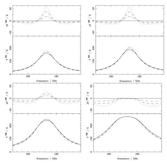
Figure 3: The effect of changing the scale height,  $h_0$ , on the brightness temperature. Top left for PWV = 0.5; top right PWV = 0.675; bottom left PWV = 1.275; bottom right PWV = 2.8 (representing the 10, 25, 50 and 75 percentile frequency values).  $h_0$  takes the values 0.5, 1.0, 1.5, 2.0 km corresponding to solid, dot-dashed, dashed and dotted lines respectively. The top plots of each panel show the difference in brightness temperature of each line compared with the solid line.
