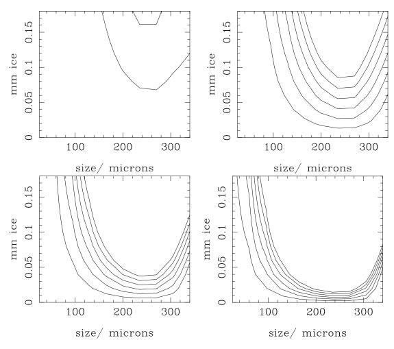
Figure 15: Contours showing the range of ice amounts and sizes that would be detectable by the radiometer channels. Top left is for channel 1; top right for channel 2; bottom left for channel 3 and bottom right for channel 4. Contour levels represent 1, 2, and 3 (4,5,6)  $\sigma$  errors expected from measuring the brightness temperature asymmetry. The asymmetry needs to be higher than the expected errors in order to be detectable.
