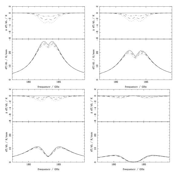
Figure 9: The effect of changing the lapse rate,  $\Gamma$ , on the sensitivity dT/dL. Top left for PWV = 0.5; top right PWV = 0.675; bottom left PWV = 1.275; bottom right PWV = 2.8 mm (representing the 10,25,50 and 75 % frequency values).  $\Gamma$  takes values -2.5, -5, -7.5, -10. K/km corresponding to solid, dot-dashed, dashed and dotted lines respectively.
