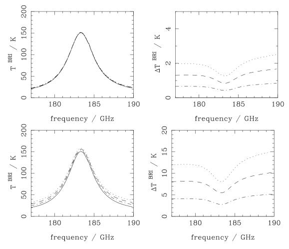
Figure 13: The impact of varying amounts of ice on brightness temperatures. The ice particles are spherical with radius 100 in the top panels, and 200  $\mu$ m in the bottom panels. Left panels show the brightness temperature, and right panels show the change in brightness temperature as a result of the ice (solid line is for no ice; dot-dashed for 0.05 mm of ice; dashed for 0.1 mm; and dotted for 0.15 mm).
