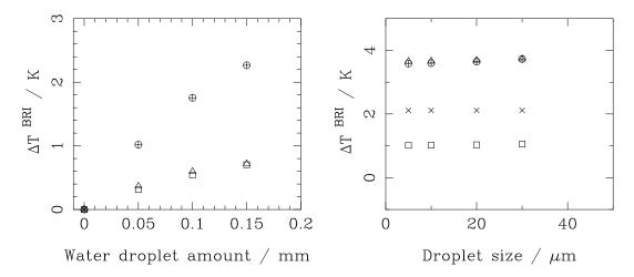
Figure 17: Left panel shows the additional asymmetry resulting from varying concentrations of water droplets of size 10  $\mu$ m. Right panel shows the asymmetry for varying sizes of water droplet and 0.1 mm of liquid water. Crosses are for channel 1, squares for channel 2, triangles for channel 3 and circles for channel 4.
