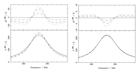
Figure 2: Bottom panels: Left: The effect of changing the pressure of 1 mm PWV at a fixed temperature of 265 K. Solid line is for 560 mb; dot-dashed for 480 mb; dashed 415 mb; and dotted, 375 mb. Right: The effect of changing the temperature of 1 mm PWV at a fixed pressure of 491 mb. Solid line is for 264.2 K; dot-dashed for 260.1 K; dashed, 256.1 K; and dotted, 252.2 K. Top panels show the difference in  $T^{\rm BRI}$  of each line compared with the solid line.
