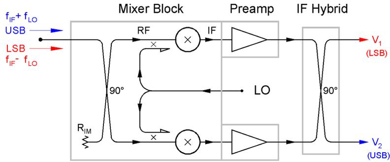
Fig. 1. Sideband-separating mixer configuration used for Band 6.
