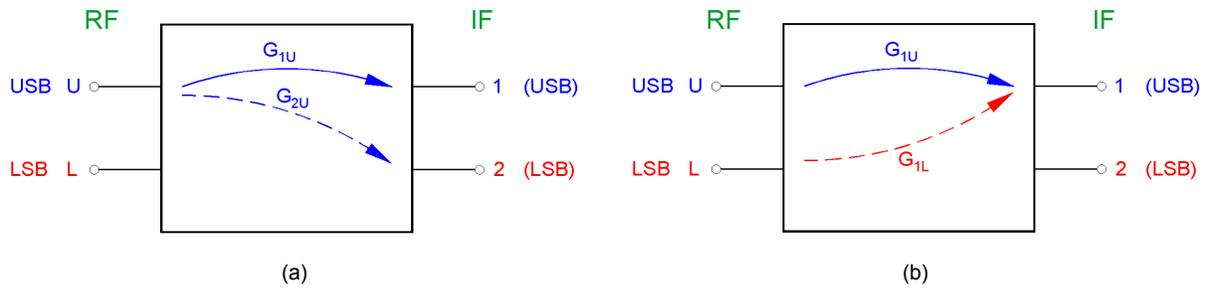
Fig. 6. Two definitions of image rejection. (a) Image rejection  $R_a = G_{1U}/G_{2U}$ . (b) Image rejection  $R_b = G_{1U}/G_{1L}$ . In the context of radio astronomy, (b) is the appropriate definition.
