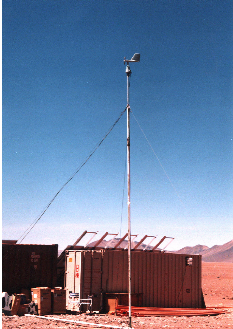
Figure 1: The N-800S anemometer installed atop an 8.0 m mast at Pampa La Bola as seen from southwest (photo as of 2000 February 6). The most significant nearby obstacles are two 20 ft containers ( 6.06 \times 2.49 \times 2.50 m) placed about 7 m to the north.
