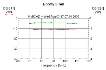
Fig. 4.  $|S_{11}|$  (red, dB, left scale) and  $|S_{21}|$  (green, dB, right scale) of a 5-mil section of WR-10 filled with Epo-Tek 301-2.
