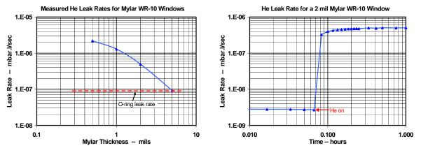
Fig. 2. He leak rates of Mylar WR-10 waveguide windows: (left) as a function of Mylar thicknesses, and (right) as a function of time for a 2 mil window.
