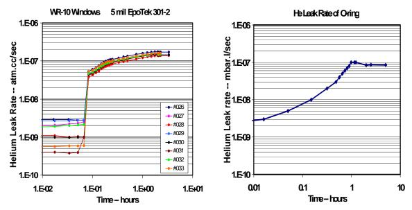
Fig. 5. Left: Helium leak rate as a function of time, for eight windows. Right: Leak rate of the O-ring. The window under test was covered with a balloon full of helium during the measurements.
