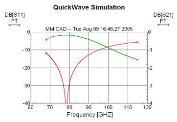
Fig. 6. QuickWave Simulation of the feedthrough assembly in Fig. 1.  $|S_{11}|$  (red, dB, left scale) and  $|S_{21}|$  (green, dB, right scale).
