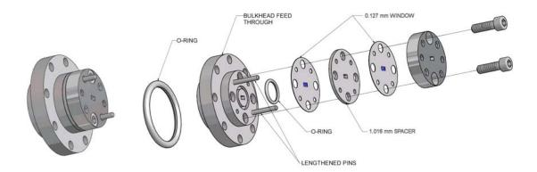
Fig. 1. Assembled and exploded views of the feedthrough. The two 0.127 mm waveguide windows are filled with epoxy. The left window, against the small O-ring, provides the vacuum seal and the second window, to the right of the 1.016 mm spacer, cancels reflections from the first.
