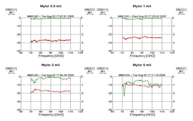
Fig. 3.  $|S_{11}|$  (red, dB, left scale) and  $|S_{21}|$  (green, dB, right scale) of Mylar sheets of several thicknesses clamped between the WR-10 waveguide flanges of an Agilent 8510 VNA.
