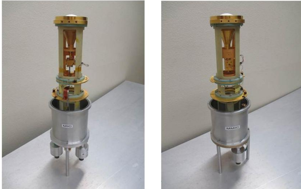
Figure 8: ARO receiver cartridges with 80nm MIC LNA (left) and 35nm MMIC LNA (right).
