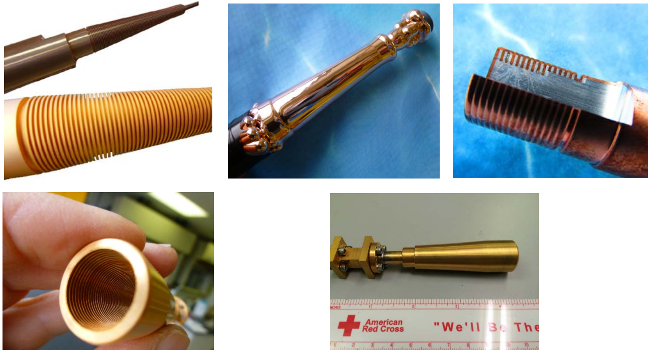
Figure 8: Stages of Feed Horn Fabrication
