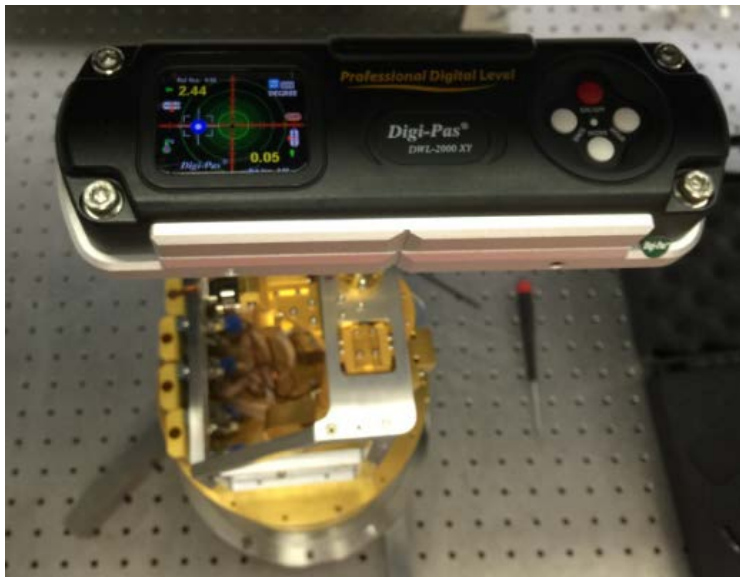
Figure 32: In-house inclinometer measurements of feed horn tilt
