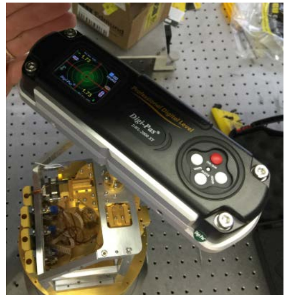
Figure 32: In-house inclinometer measurements of feed horn tilt
