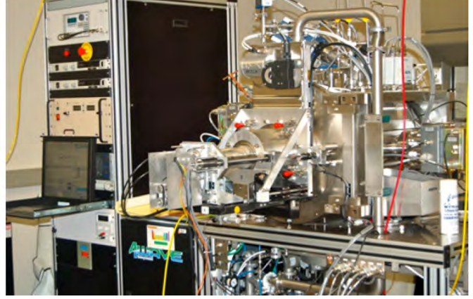
Figure 2.2: Fig. 4. Left: Schematic of Reactive Bias Target Ion Beam Deposition system; Right: Photograph of the UVA 4-Wave RBTIBD tool that can accept up to 100 mm diameter wafers.
