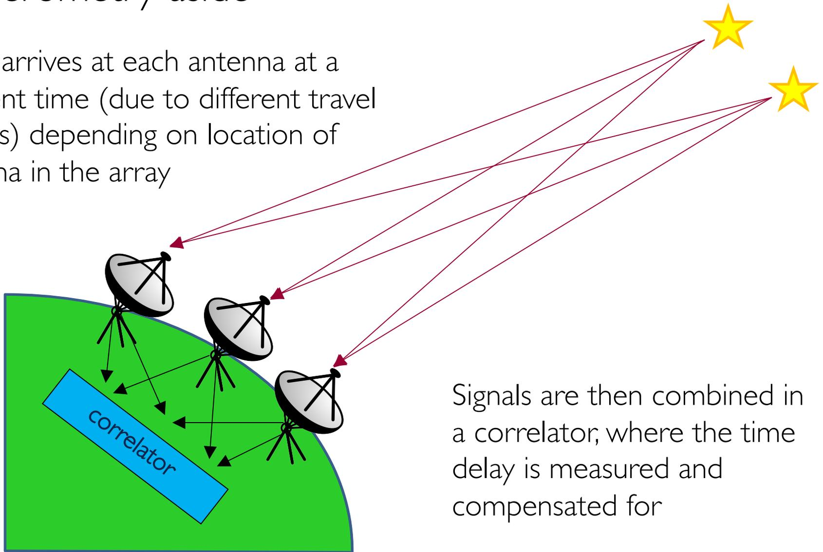
Signals are then combined in a correlator, where the time delay is measured and compensated for
