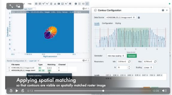
If there are multiple images loaded in append mode, users may use the "Data Source" dropdown to select an image as the data source of contour calculations. If the state of the "lock" button is locked, the image viewer will show the selected image as a raster image and the image slider in the animator widget will be updated to the selected image too. To disable this synchronization, click the "lock" button to set the state to unlock.
