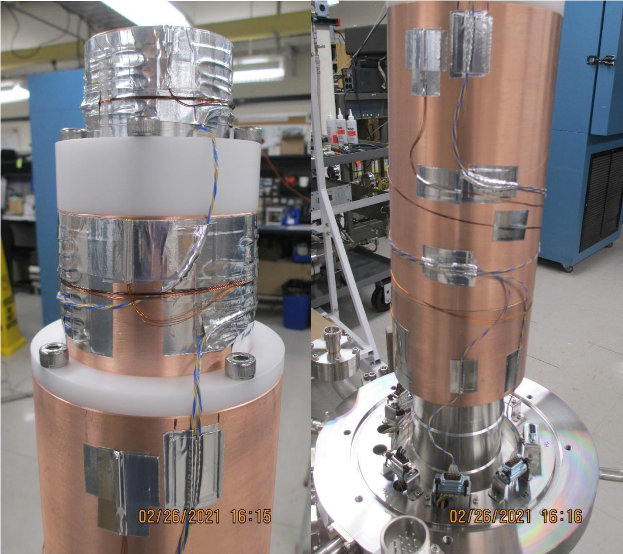
Picture 15: Installation of Temperature Sensors & Headers
