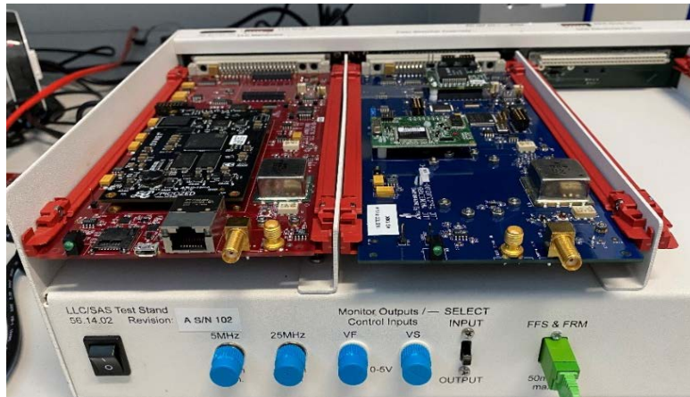
Fig 5: The new LLC Mainboard (left), and the existing baseline one (right).
