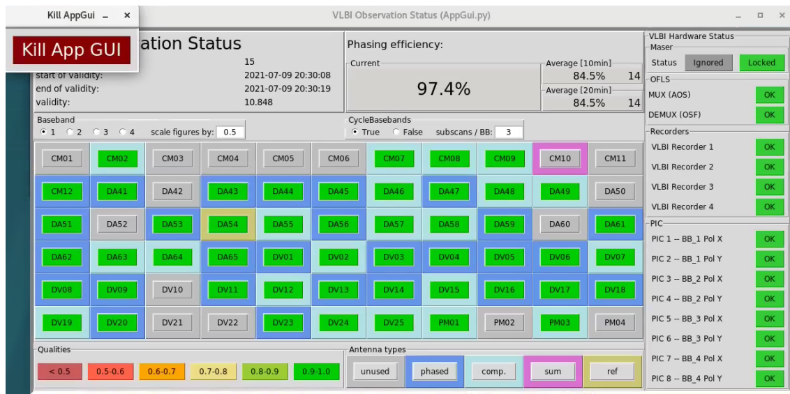
Figure 30: A sample of the main panel of the updated APP GUI ( AppGUI ) tool, which is used by the ALMA operator during VOM observations to monitor the phased array.
