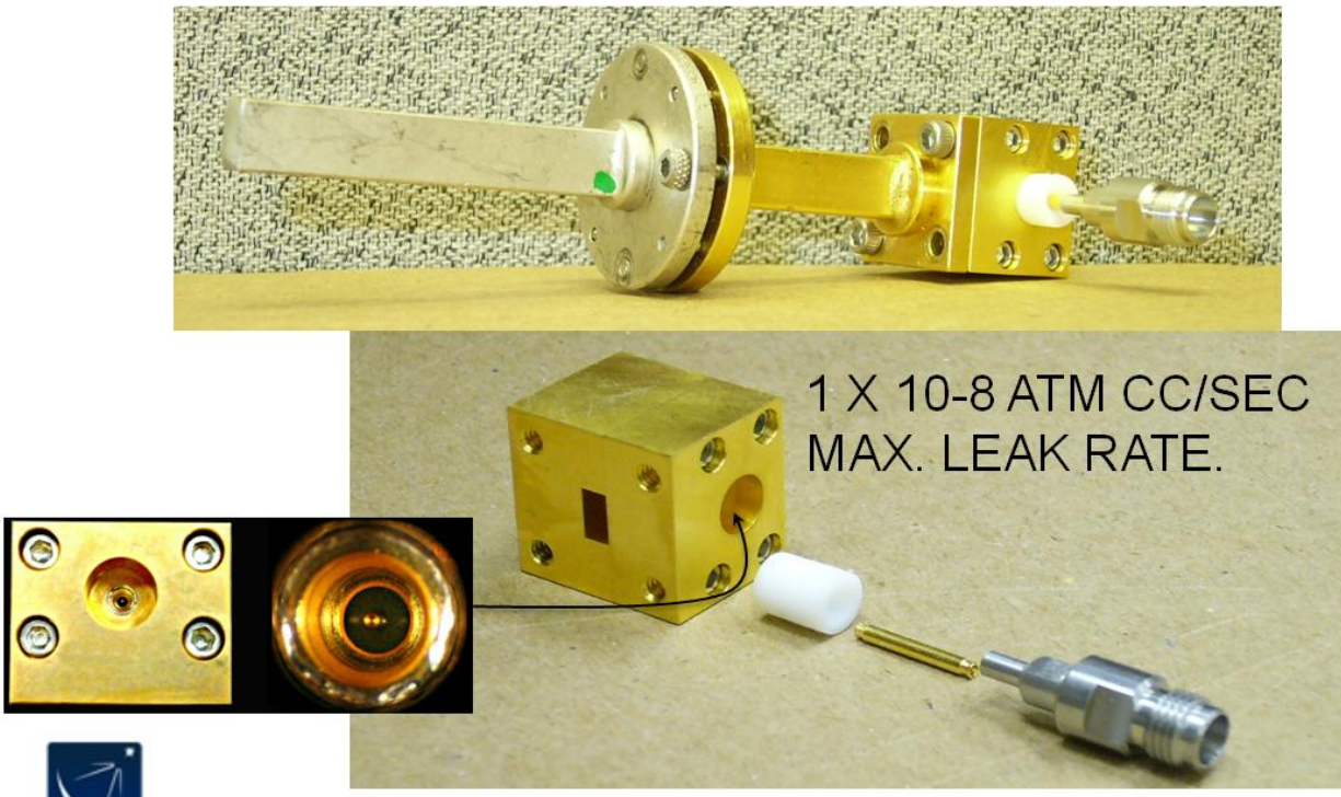
Figure 50: Hermetic Blind-Mating WR22-G3PO-V Connector
