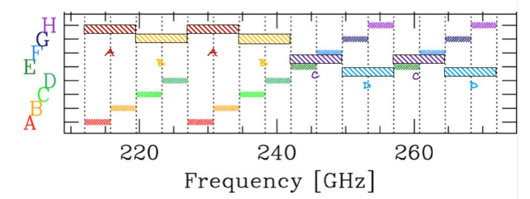
Upgraded ALMA Correlator needs *only four* settings to cover Band 6; currently *eight* tunings (Lettered, left) are needed to cover the frequencies of the [C II] line at redshifts of 6 to 8 in the ALMA ASPECS spectral scan of the Hubble UltraDeep Field.
