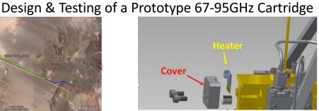
Band 3 CCA Heater Installation for **Deflux Operation**
