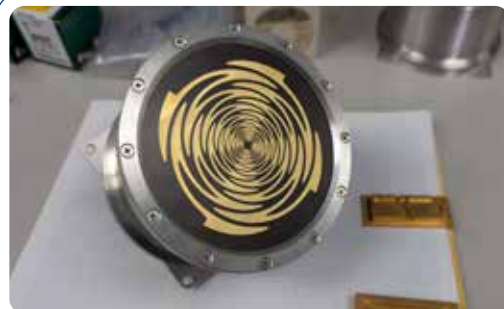
Above: The first redesigned ASM-2 Sinuous Antenna on the bench at the Central Development Lab (CDL) in Charlottesville, VA. (Photo: US NSF/AUI/NSF NRAO)
