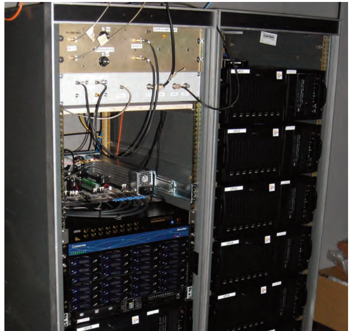
Fig. 12: The Green Bank Ultimate Pulsar Processing Instrument (GUPPI) is a pulsar detector built with off-the-shelf hardware and custom software.
