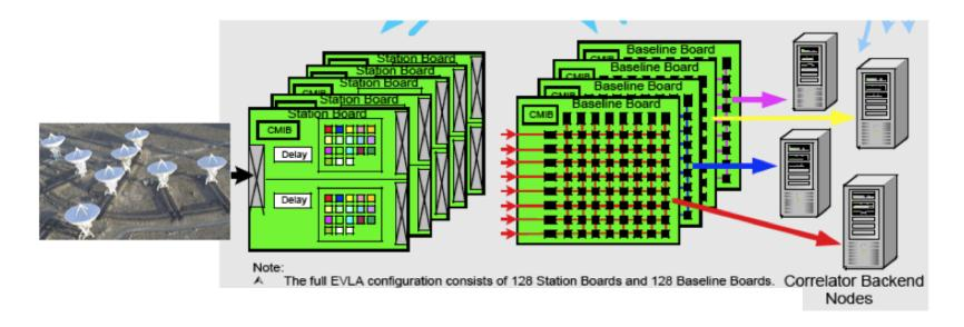
16 GHz/ant split into 4 x 2 GHz/pol'n (Baseband pairs) Station Boards: split into 64x128 MHz/pol'n (Sub-band pairs)
