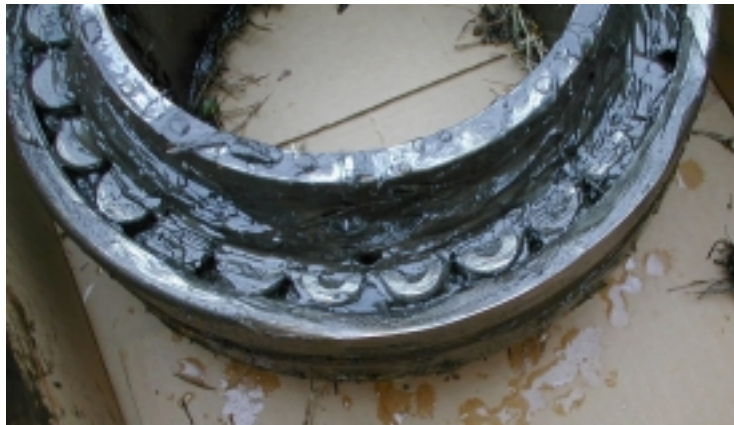
Figure 1: Failed Azimuth Bearing
