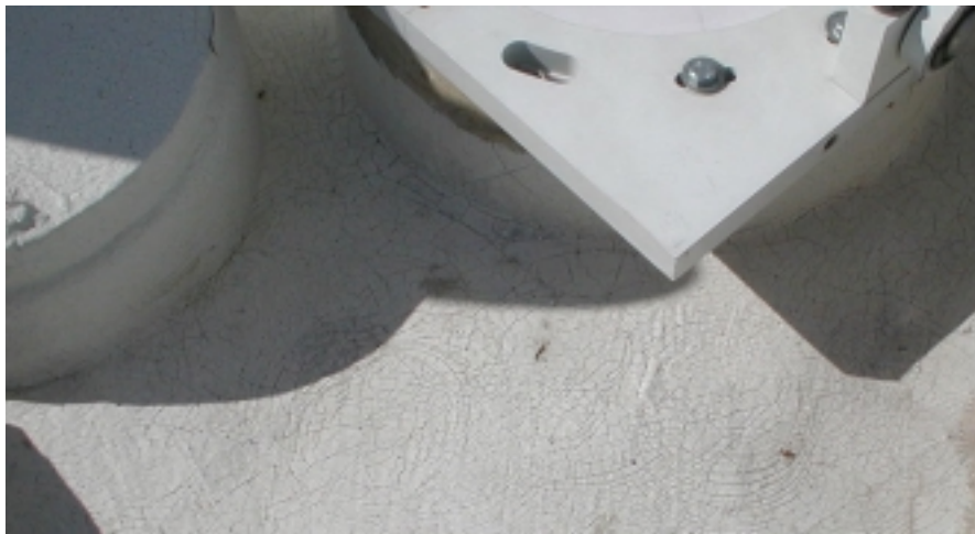
The feed cone finish is checked
