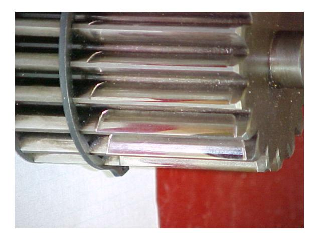
The photograph below shows that the sun gears in Az#1 gearbox are worn on the counter clockwise rotation side while the sun Gears in Az#2 gearbox are worn on the clockwise side. The sun gears show very little wear on the opposite side. This uneven wear is probably due to the 30% servo preload used to reduce backlash. If this is the case, we should be able to extend the life of the gears by reversing the direction of the preload or swapping the gears from one gearbox to another.
