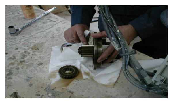
Azimuth #1 gearbox pre-load inspection.
