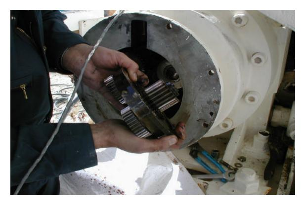
Elevation gearbox #1 pre-load inspection showed very little signs of wear. Both gearboxes oil was changed and several flow gauges were replaced.
