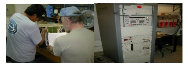
The ACU power supply upgrade was completed. During the ACU retrofit 6 bad TB2 crimps were found and repaired. The AZ synchro was repaired.
