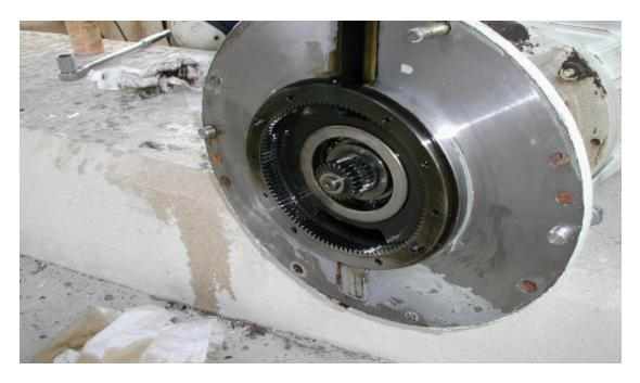
Azimuth #2 gearbox pre-load inspection. Both gearboxes showed very little signs of wear. Both gearboxes oil was changed and several flow gauges were replaced. A gearbox oil seal was replaced on AZ #1.
