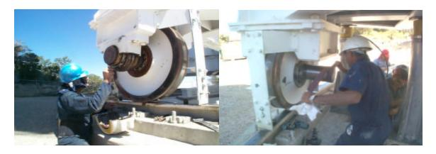
AZ wheel bearings were inspected. AZ #2 idler bearing was replaced. No popping or grinding noises were heard from the AZ bearings or gearboxes.
