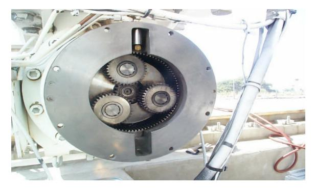
Azimuth #1 gearbox pre-load inspection
