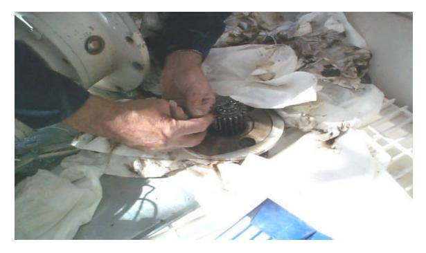
Steve measures ~.002 of wear with a feeler gauge showing EL #2 gearbox is in good condition. Both EL gearboxes oil was changed. Fish eyes and flow gauges were also cleaned. EL #1 gearbox was not opened for inspection.
