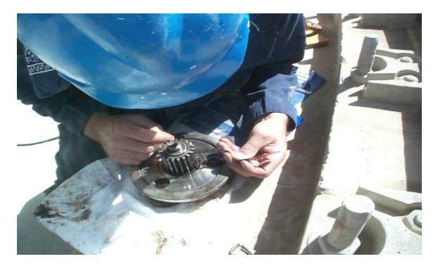
Steve measures ~.002 of wear with a feeler gauge showing AZ #1 gearbox is in good condition. Both AZ gearboxes oil was changed. Fish eyes and flow gauges were also cleaned. AZ #2 gearbox was not opened for inspection.
