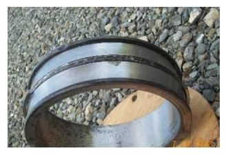
The original bearing's inner ring center guide flange was fractured. According to engineers at Torrington Bearing, this kind of fracture is due to excessive thrust load on the bearing.
