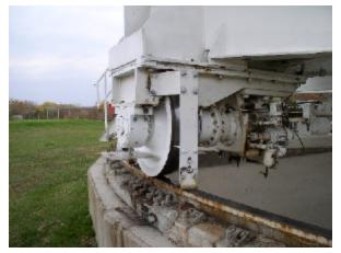
The new wheel/axle assembly was installed and aligned. After two days of operation, the following alignment parameters where recorded for the new axle/wheel assembly. The antenna rotated smoothly without popping sounds.
