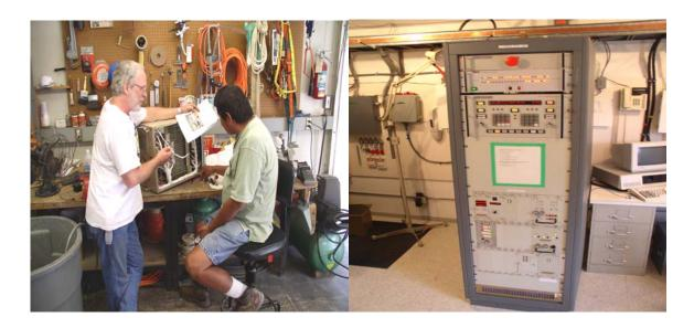
DJ and Nelson retrofitted the ACU with the new power supply upgrade.
