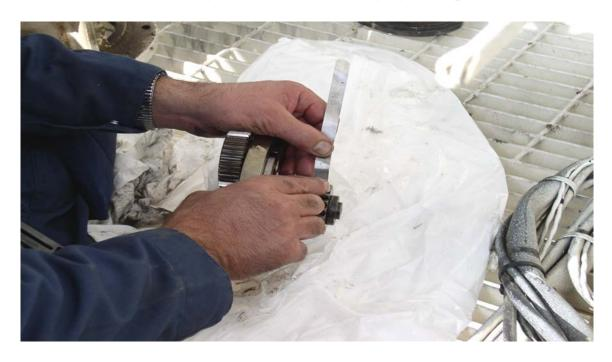
Steve measures ~.0015 of wear with a feeler gauge. Elevation #1 gearbox is in good condition. Both elevation gearboxes oil was changed. Fish eyes and flow gauges were cleaned. Elevation #2 was not opened for inspection.
