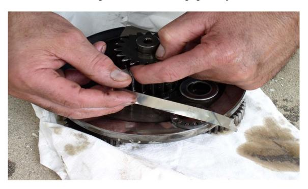
Steve measures ~.001 of wear with a feeler gauge. Azimuth #2 gearbox is good condition. Both azimuth gearboxes oil was changed. Fish eyes and flow gauges were cleaned. Azimuth #1 was not opened for inspection.
