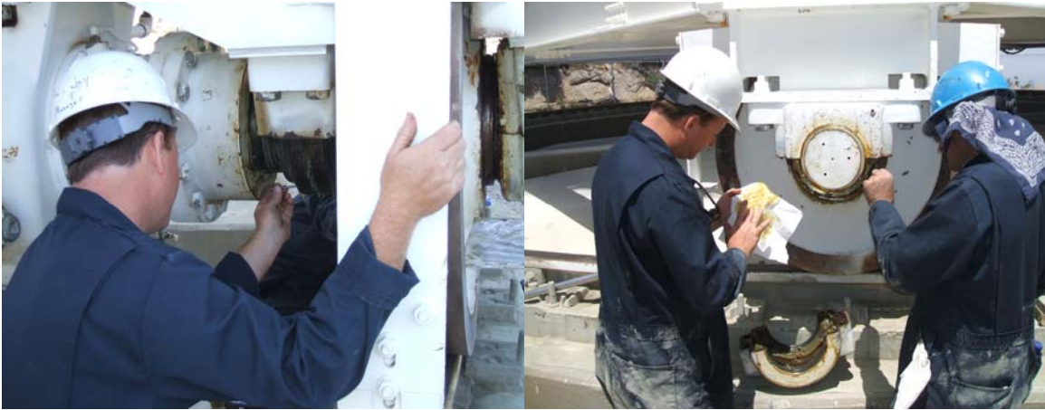
Azimuth wheel bearings were inspected, none were replaced.
