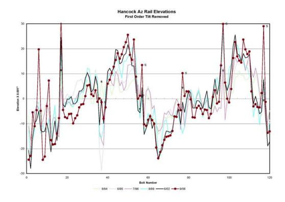
Splices at bolt numbers, 17, 97 and 117 are failing. Page 10
