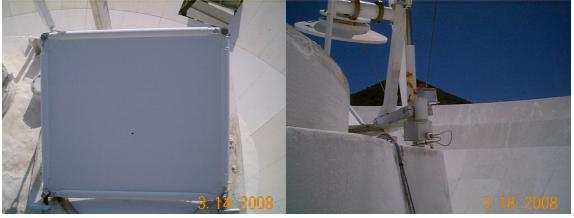
Dichroic reflector is in good condition. Ellipsoid reflector is in good condition. Dichroic reflector actuator operates correctly.
