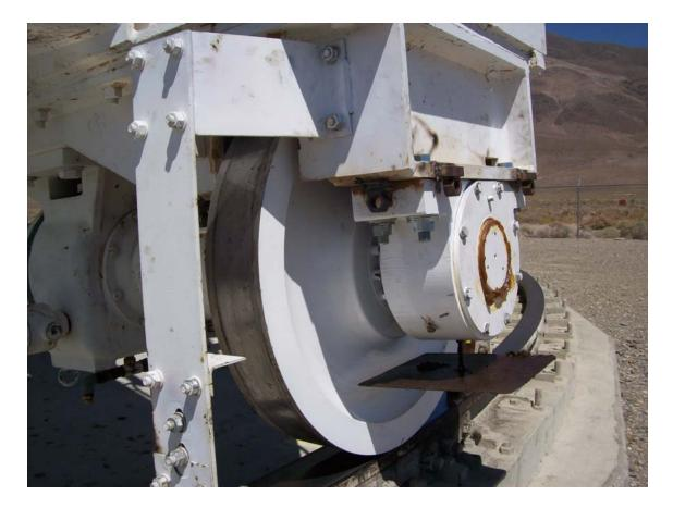
Azimuth #1 Wheel assembly was replaced. The new drive wheel assembly rotated smoothly without any popping or grinding noises.
