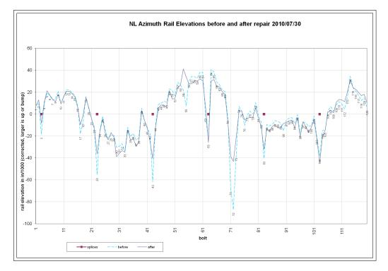
Figure 13: Rail height before and after repair
