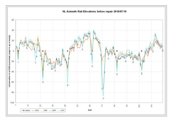
Figure 1: Rail height since last repair
