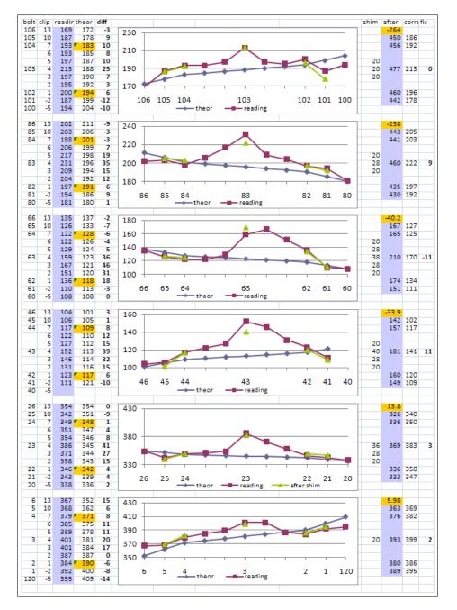
Figure 12: Low spots at splices and shimming attempts
