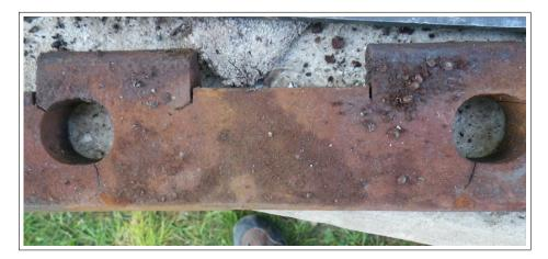
Figure 8: Splice bar typical cracks at North Liberty antenna
