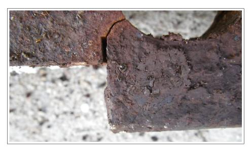
Figure 9: Splice bar typical cracks at North Liberty antenna
