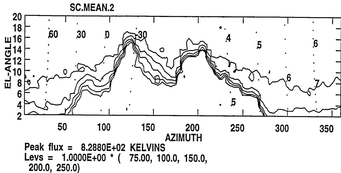
Figure 9: St. Croix horizon data; contours at  $T_{sys} = 75, 100, 150, 200, 250$  K. Sidereal tracks for various delineations are indicated; the numbers on the left indicate the declination, the numbers on the right hour angles. These data are from only the first SC raster; the second raster had data problems and was not used.
