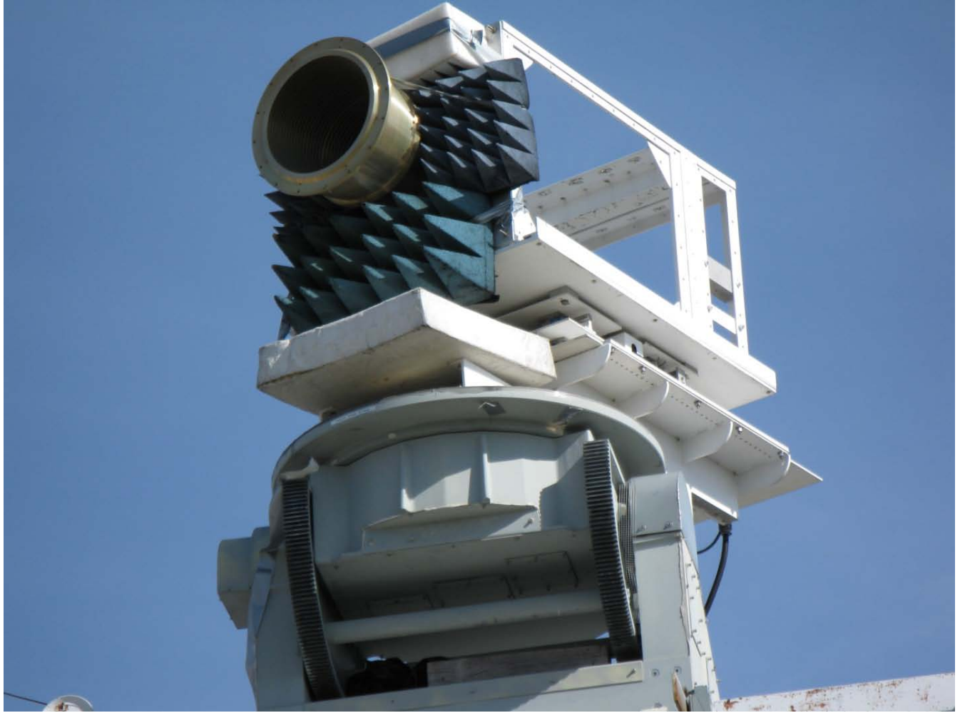
Figure 2. Feed horn on the Green Bank outdoor range tower.
