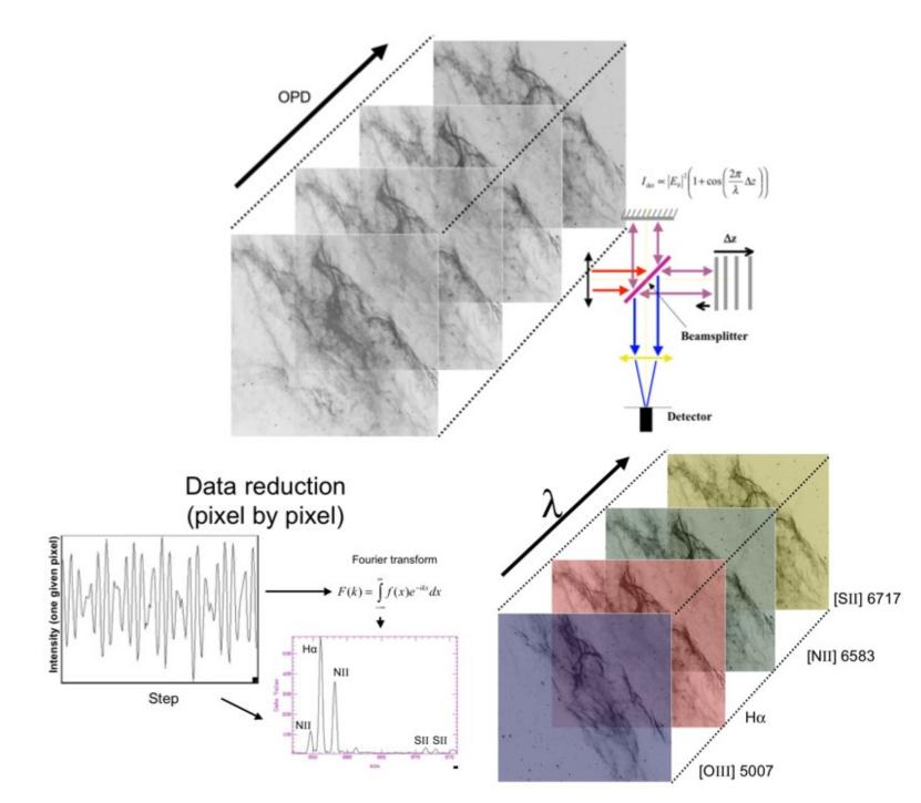
The hyperspectral datacube is constructed by sampling the interferogram of each pixel by varying the optical path difference (OPD). Afterwards, this can be Fourier-transformed into the desired spectrum at each pixel.
