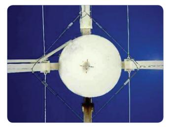
Four Modified J-Pole feeds on a VLA antenna.
