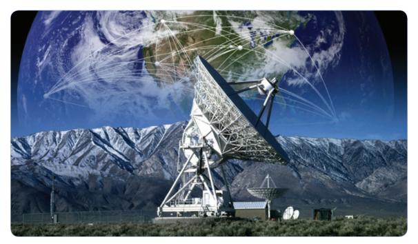
new receivers on all 28 antennas, along with a new digital data transmission system and a new Wideband Interferometric Digital Architecture (WIDAR) correlator, provide superb spectral resolution and fidelity over very wide instantaneous bandwidth, enabling astronomers to make full-beam images with very high spatial resolution and dramatically improved continuum sensitivities from 1-50 GHz.
