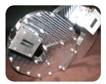
An OMT designed and fabricated by the CDL for the Green Bank Telescope pulsar receiver.
