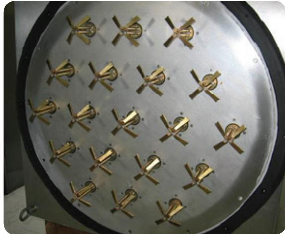
*Nineteen element dual-polarization Phased-Array Feed with cryogenic SiGe HBT LNAs. Measured Tsys of 35K on the Green Bank 20m telescope.*
