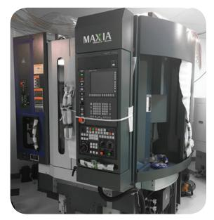
Above: The new Matsuura LX-160 precision milling machine in the CDL machine shop adds the capability to manufacture sub-mm wave assemblies with stringent tolerance requirements.
