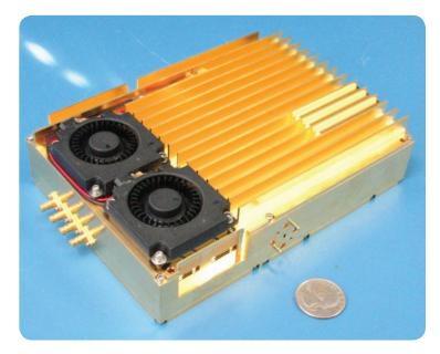
The IRD group also procured the necessary hardware to implement an unformatted serial link operating at 10 Gbps over 40 km of fiber. Preparations are also underway to demonstrate its operation. This is the longest distance over which this has been ever attempted. Confidence level for a successful test is very high, and this will have positive implications for the ngVLA.
