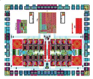
Above: Physical layout of the 10 Gbps serial-ADC custom integrated circuit. Below: Figure: A proof-of-concept deep rejection filter.
