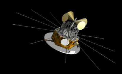
Ball has demonstrated capability in constructing RF quiet S/C as evidenced by DARPASat, which beat MIL-STD-461E standards by 44 dB. Technology advances since DARPASat will further quiet the DARE S/C by another 10 dB.
