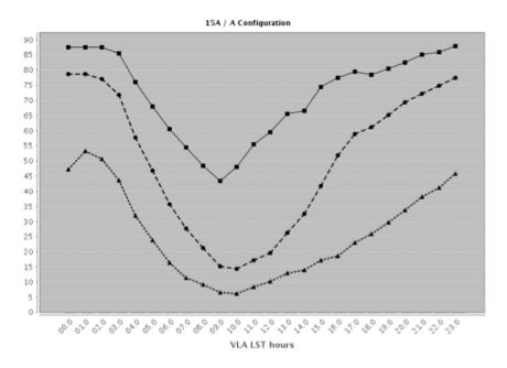
**BnA configuration:** Estimated science time available per LST hour is shown by the solid black line for all frequencies, the dashed line for K-band conditions, and dotted line for Q-band conditions.
