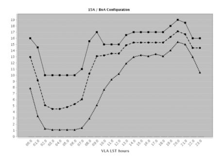
**B configuration:** Estimated science time available per LST hour is shown by the solid black line for all frequencies, the dashed line for K-band conditions, and dotted line for Q-band conditions.
