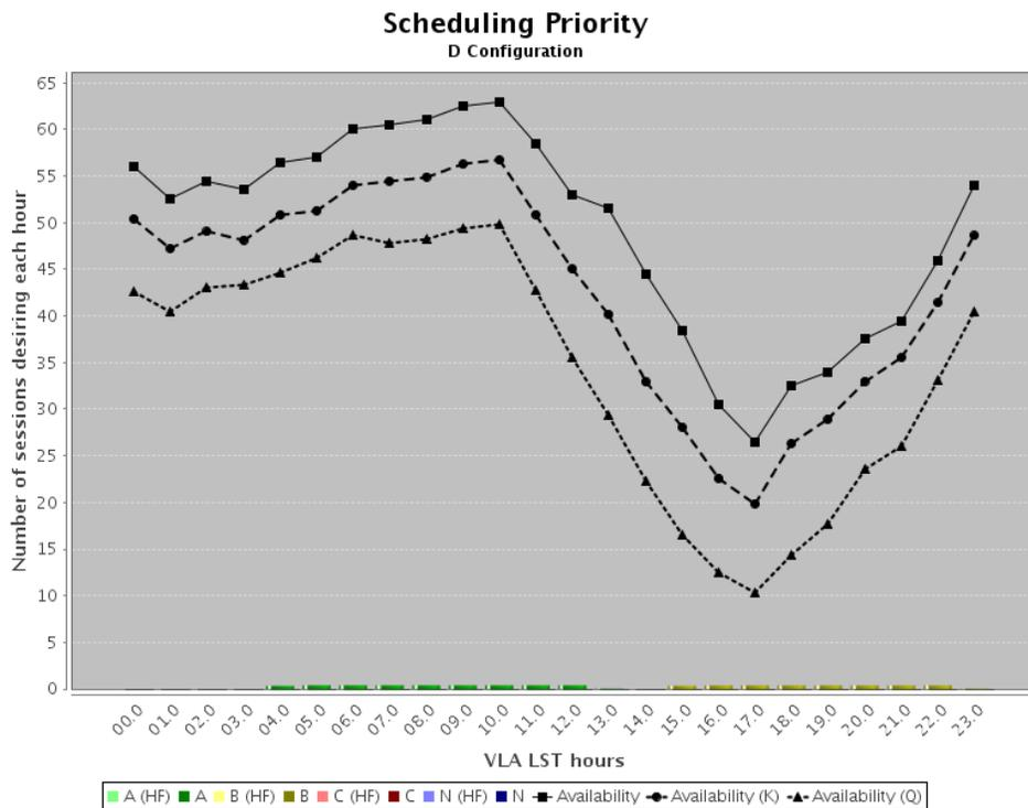
**DnC configuration:** Estimated science time available per LST hour is shown by the solid (upper) black line for all frequencies, the dashed (middle) line for K-band conditions, and dotted (lower) line for Q-band conditions.
