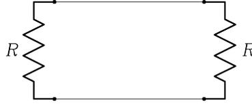
Fig. 7.— Two resistors connected by a lossless transmission line of length  $a \gg \lambda$ , the longest wavelength of interest. In equilibrium, the transmission line can support only those standing waves having zero voltages at the ends; other modes are suppressed by the lossy resistors.
