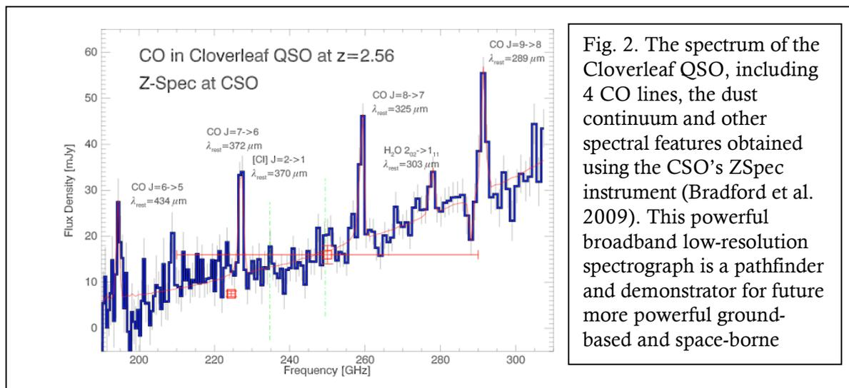
Fig. 2. The spectrum of the Cloverleaf QSO, including 4 CO lines, the dust continuum and other spectral features obtained using the CSO's ZSpec instrument (Bradford et al. 2009). This powerful broadband low-resolution spectrograph is a pathfinder and demonstrator for future more powerful ground-based and space-borne
