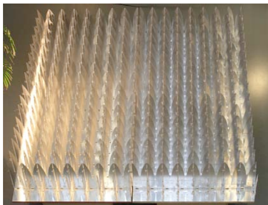
Figure 7 — (Left) Example “checkerboard” phased array feed (PAF) for the Australian SKA Pathfinder project (Photo credit: David McClenaghan, CSIRO). PAFs will greatly increase the survey speed of the SKA. (Right) An alternative approach is to use phased arrays to sample the sky directly, as in European efforts to develop aperture array tiles (courtesy SKADS project).
